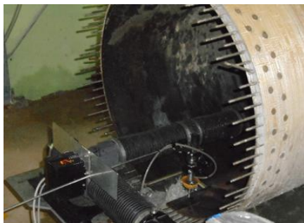
Equipment for cutting of Composite Hardware (used canister)
