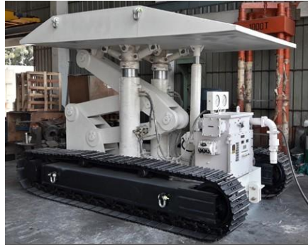
Heavy-duty 500t SAGES with a remote radio-controlled and digital display system
