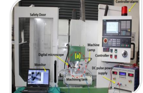
Hybrid micro machining technology using \mu -ECM and \mu -EDM processes
